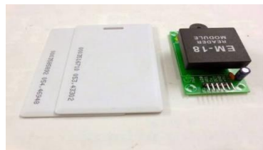
Figure 2 RFID Reader and Tag
