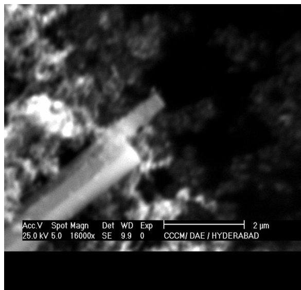
Figure 1 SEM image of Flame synthesized nano carbon
